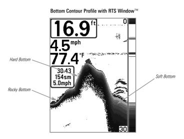
The sonar returns from the bottom, structure, and fish can be represented as **Inverse**, **Structure ID®**, **WhiteLine**<sup>TM</sup>, or **Black** (Bottom Black). See **Sonar X-Press Press Menu**: **Bottom View** to set the bottom view.
